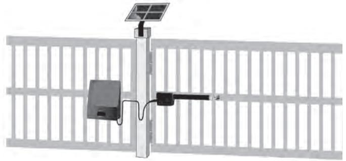
When deciding where to mount the control box remember the actuator cable is 8 feet in length. If possible, mount the control box in a location that will allow the cable to be neatly routed. If it must be longer than the 8 feet, see Splicing Actuator Cable Step. Also avoid choosing a mounting location that is near sprinklers.
