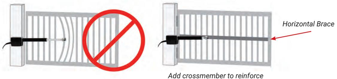
Avoid mounting actuator on bottom rail of gate. Unit will be more likely to be damaged by flooding and will be difficult to service and adjust.
