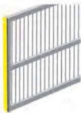
**Zone A** - Leading edge of gate where it meets a 2nd gate, stop post or passes a column or post corner. - recommended monitored entrapment protection type is B2 contact sensor or equivalent.
